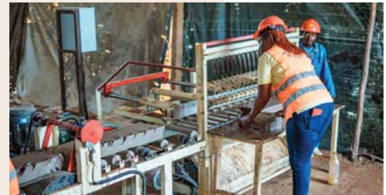
Revolution in brick making: the new motorised brick-making machine introduced by Enabel, transforming production efficiency at Optima Clays Ltd.
